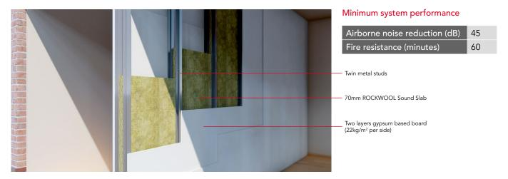
4. 'Change of use' separating wall - Independent panel to existing masonry wall
